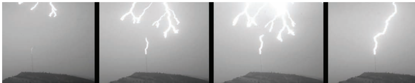
Figure 2. Selected frames from a Phantom high speed camera at 7200 frames per second showing a network of negative stepped leaders approaching a hilltop as an upward leader from a radio tower prepares to attach, completing the circuit with the upward return stroke.
